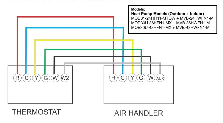
WIRING TO CONDENSER NOT SHOWN
